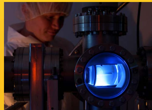
Growth of thin film by generating plasma on source material.
