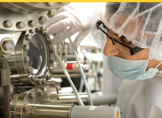
Physics graduate student working on an ultra-high vacuum molecular beam epitaxy (MBE) system used to grow thin films.
