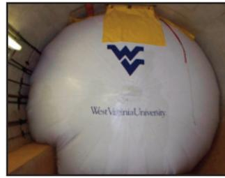
First RTC prototype for low inflation pressure
